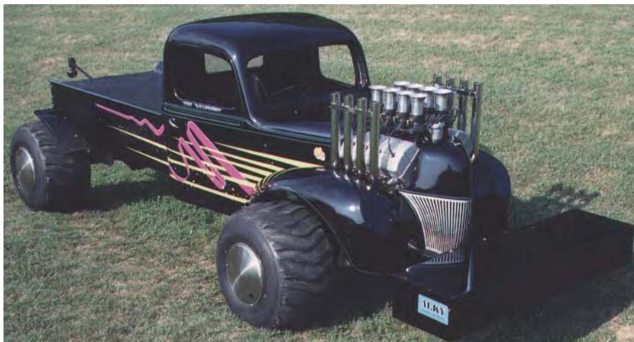
Dave Willoughby's 4-wheel drive pull truck, 700 CID Ford A/R Hemi with constant flow metering
