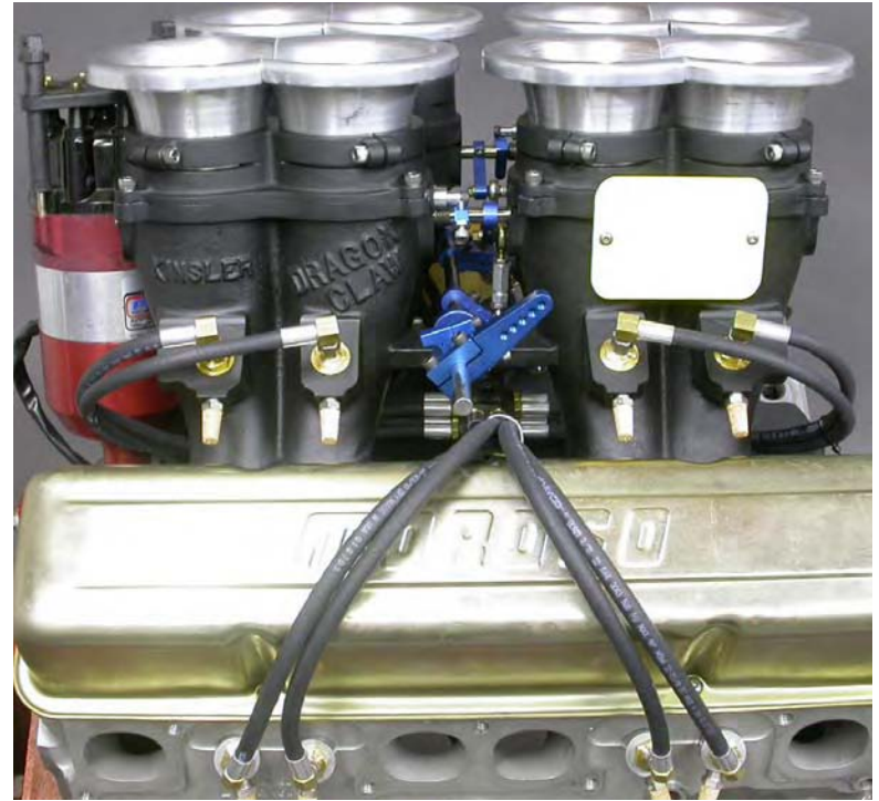
Kinsler Dragon Claw manifold with optional Jackshaft linkage kit and 16 nozzle system
