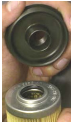
Element is o-ring sealed to endcap
