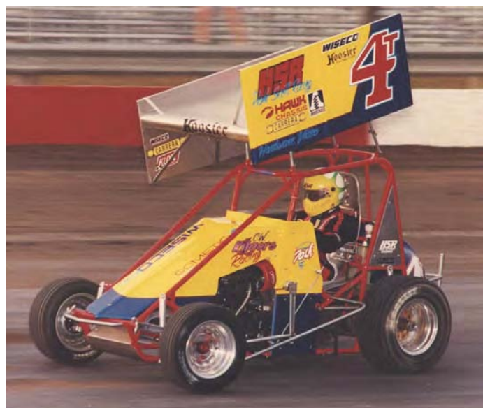
Hank Scott Racing (HSR) 1100cc oil cooled Suzuki engined Mini-Sprint Oval Track Car. Kinsler modular motorcycle injection assembly (see Page #44) with constant flow metering
