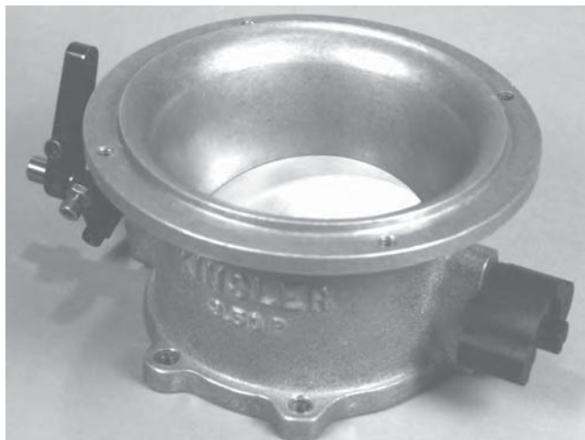
3.5P throttle body with TPS boss installed
