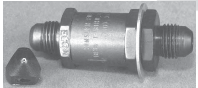
Economizer Valve has a small metering orifice drilled in the center of the poppet make certain it stays clean
