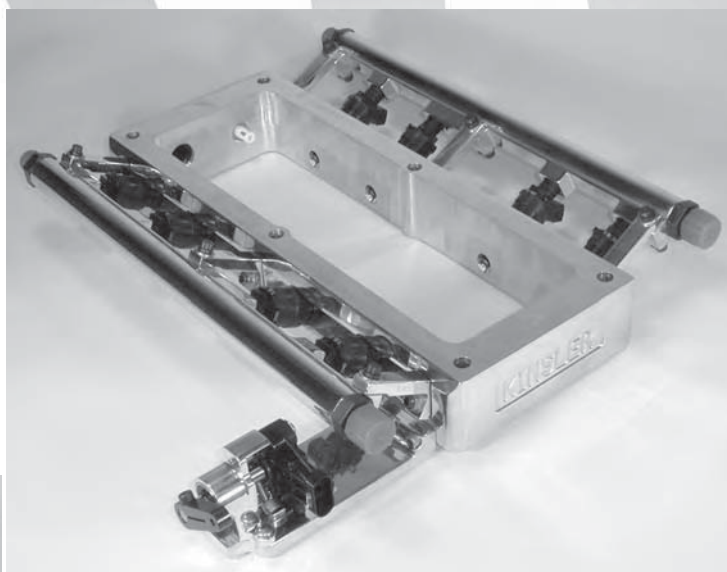
Open style adapter #16951, fuel rails, 8 injectors, remote TPS adapter
