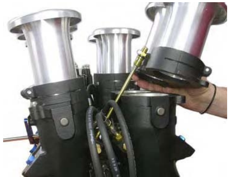
Change 5 1/2" nozzles without removing manifold from engine
