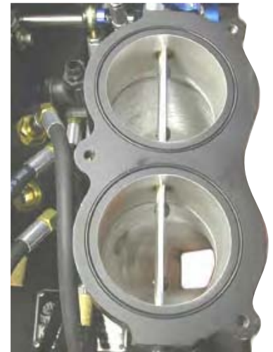
O-ring seal for manifold to ramtube adapter and backcut throttle shaft
