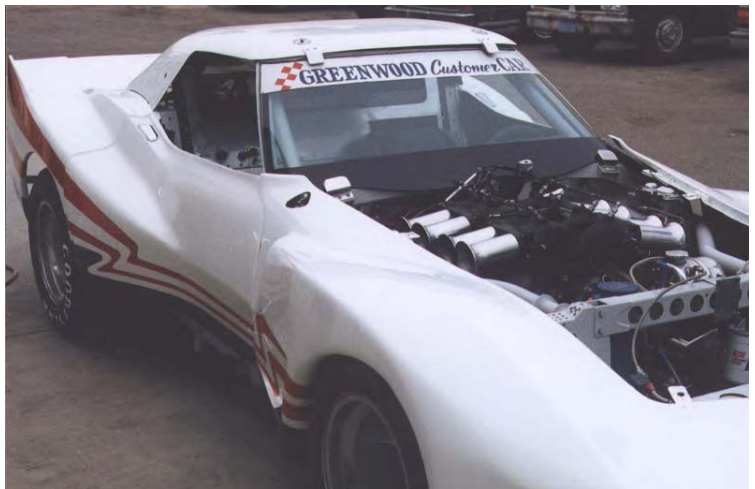
Kinsler cross-ram big block Chevrolet manifold on Greenwood IMSA Corvette using Lucas mechanical timed injection
