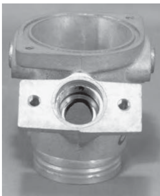
Closeup of universal boss detail in Kinsler MC-180 throttle body
