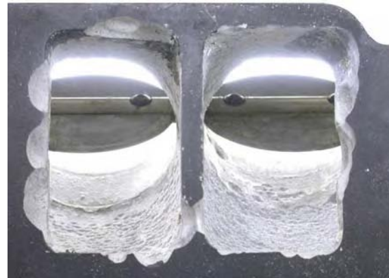
Magnesium manifold runners heavily corroded by liquid methanol left in for one week. The engine broke an inlet valve rocker arm.... since the inlet valve didn't open, the alky accumulated
