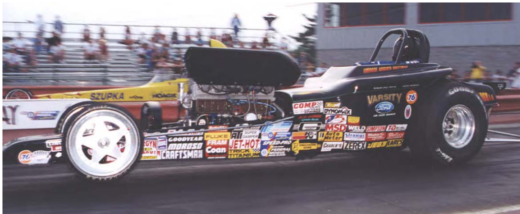
Ambrose/Argenta/Huettman/Varsity Ford's NHRA Competition Eliminator I/A record holders for E.T. (7.92 - 9/99) and M.P.H. (163.65 - 8/99) using a Kinsler fuel system on 300 cubic inch 6-cylinder in-line Ford
