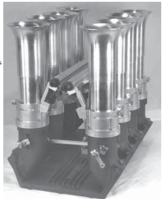
EFI injectors and fuel rails installed on dual 4-barrel manifold for big block Mopar
