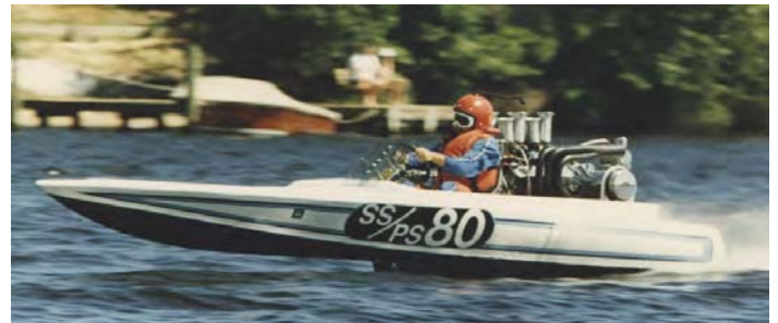
Jim Nader's 5-time National Champion Pro Stock flat bottom drag boat. 500 CID big block alky burning Chev by Mickey Marollo Racing Engines. Kinsler constant flow fuel injection system.
