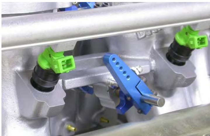
Big block Dragon Claw jackshaft linkage kit, pulls front to rear
