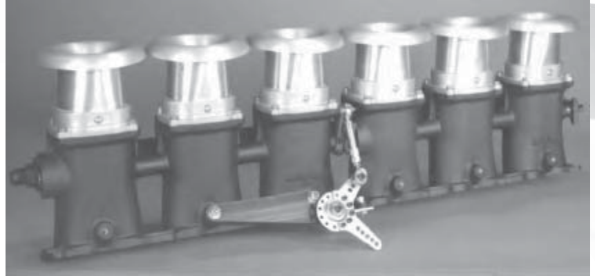
Manifold assembled from two three-cylinder castings
