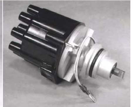
Distributor head with .165" thick tang drive
