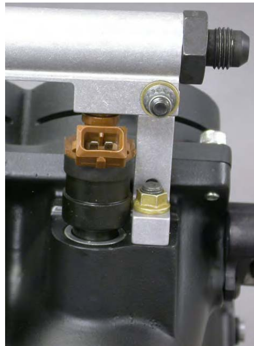
For use with electronic fuel injection, Kinsler extruded aluminum fuel rails installed
