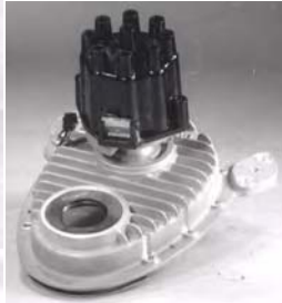
3/8" hex drive head on front cover, driven by spud bolted to camshaft
