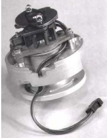
Magnetic pickup with advance weights
