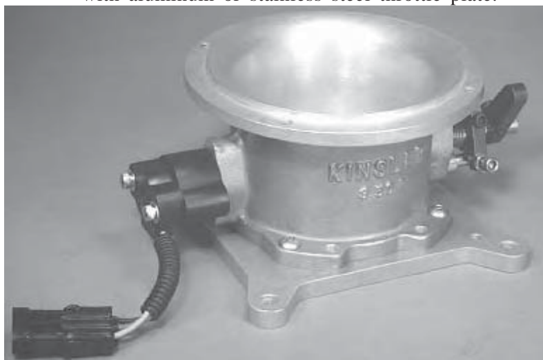
3.5P throttle body installed on 4150 Holley carb adapter plate
