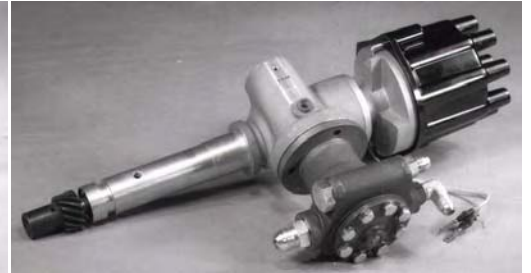
Tang drive head installed on right angle drive
