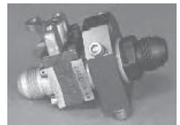
Pin removed, valve snaps closed
