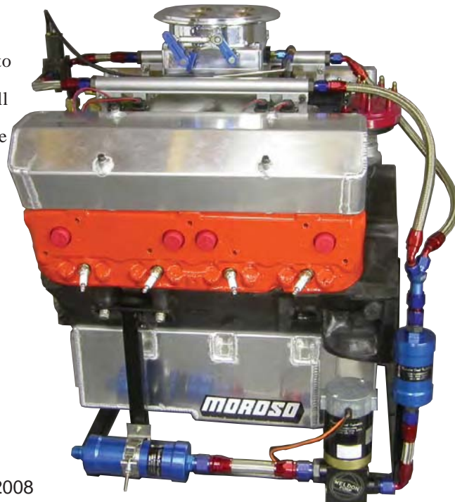
45 micron Mega Monster Mesh inlet filter, Weldon pump, 10 micron Monster Mesh outlet filter on 4-barrel throttle body system
