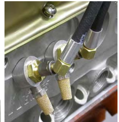
45 degree hose end on 'down' nozzle
