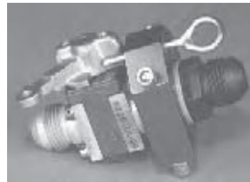
Pin installed, valve is open
