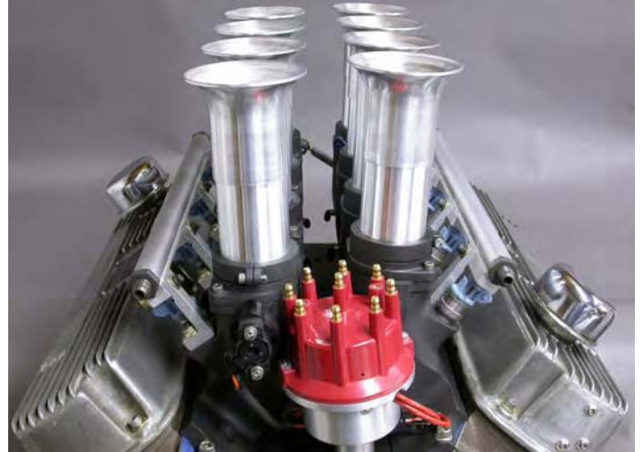
Windsor port profile with 2.0" throttle and EFI for street application
