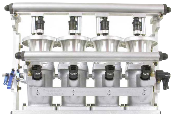
Honda F-series ITB, custom designed for Bisimoto Engineering
