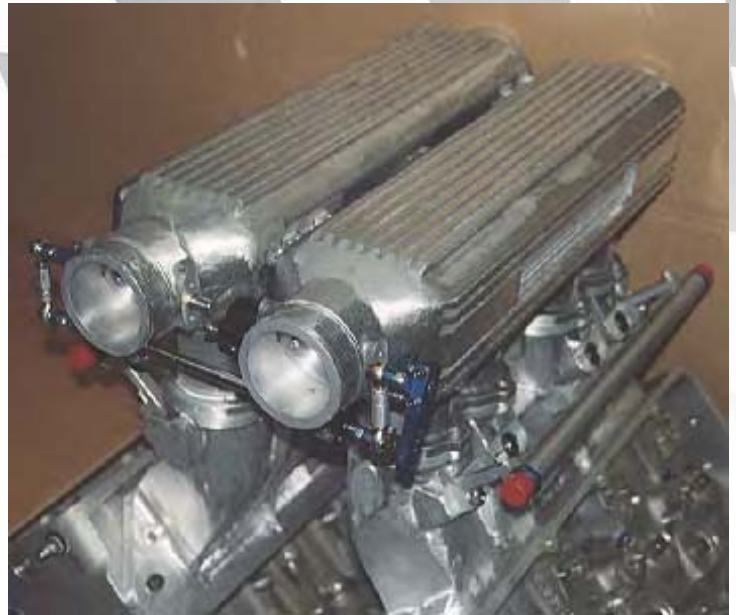
Logs with 2.5" throttle plates, on Kinsler 3-piece Pontiac Pro-Stock manifold with aluminum fuel rails
