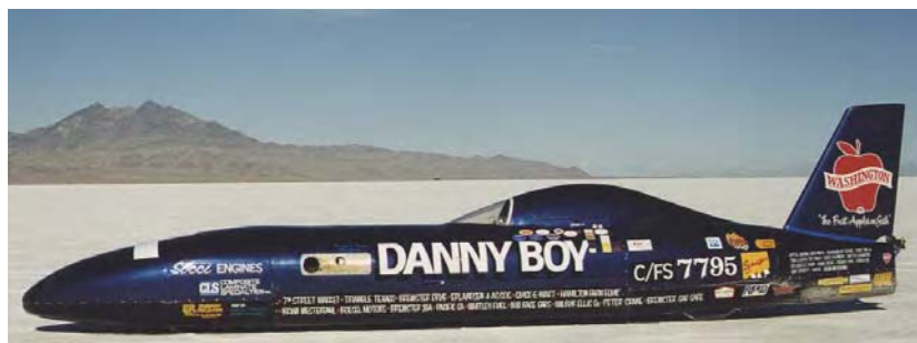
Danny Boy Land Speed Streamliner owned by Richard Thomason and Ed Tradup. Powered by a small block Chevrolet V8 with Kinsler 3-piece Dart/Buick manifold equipped with F.A.S.T. EFI system
