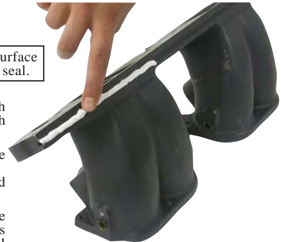
Push silicone into grooves
