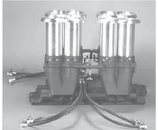
'XTRA-LIGHT' 2 5/8" throttle size manifold, nozzle bosses removed from castings, optional port profile- All Pro 285 stage II
