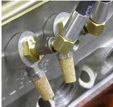
Nozzle lines with 45 degree ends and aluminum banjos with air filters for 'down' nozzles in cylinder head
