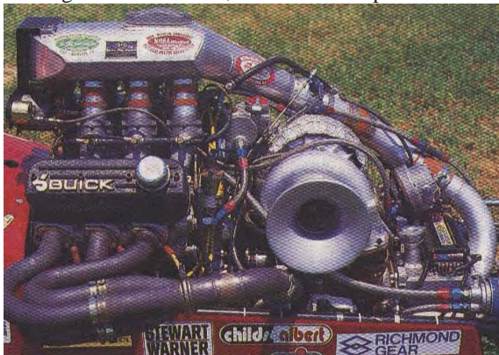
Hill and William's turbocharged Buick V6 with constant flow metering
