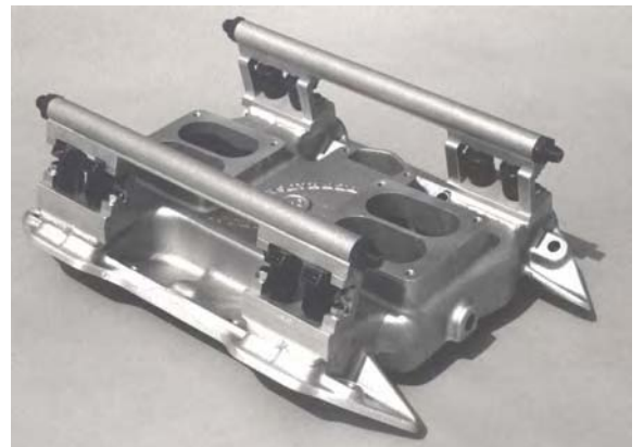
EFI injectors and fuel rails installed on dual 4-barrel manifold for big block Mopar
