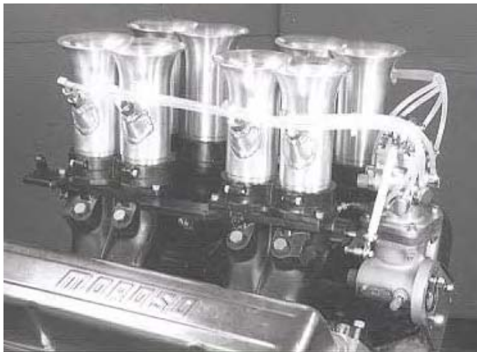
Small block Chevy manifold with Lucas Mechanical fuel injection, note the nozzle bosses in ramtubes, see Page # 54
