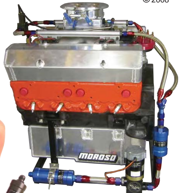
Monster Mesh inlet and outlet filters, Weldon pump, K-140 pressure relief valve - a bullet-proof combination
