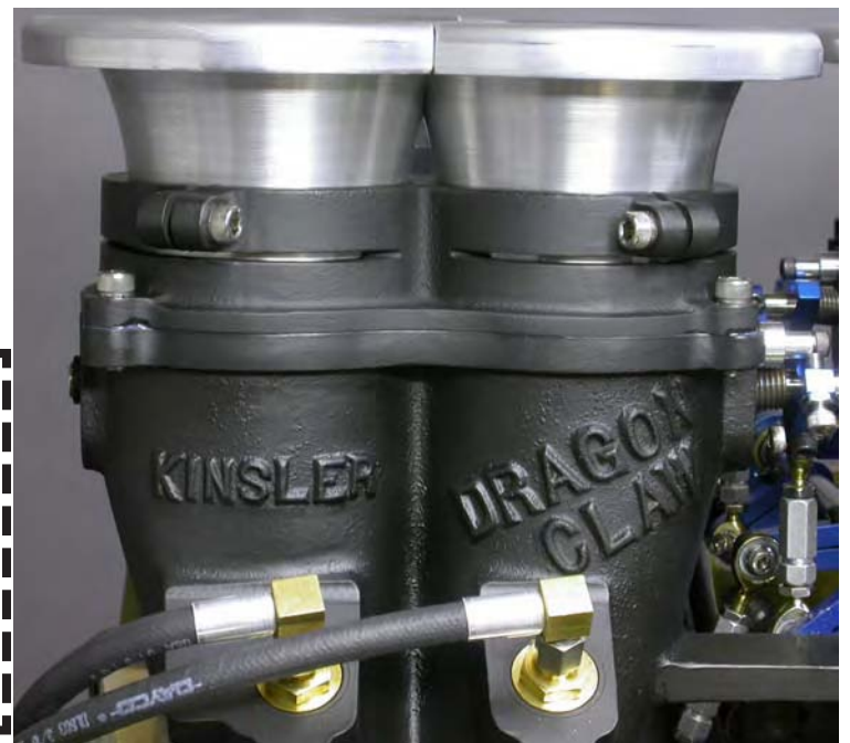
Kinsler Dragon Claw manifold with optional Jackshaft linkage kit and 16 nozzle system
