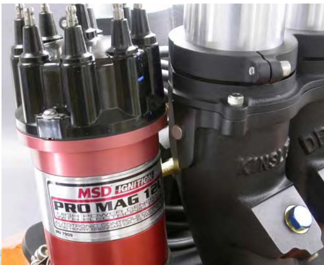
Runners machined for magneto clearance
