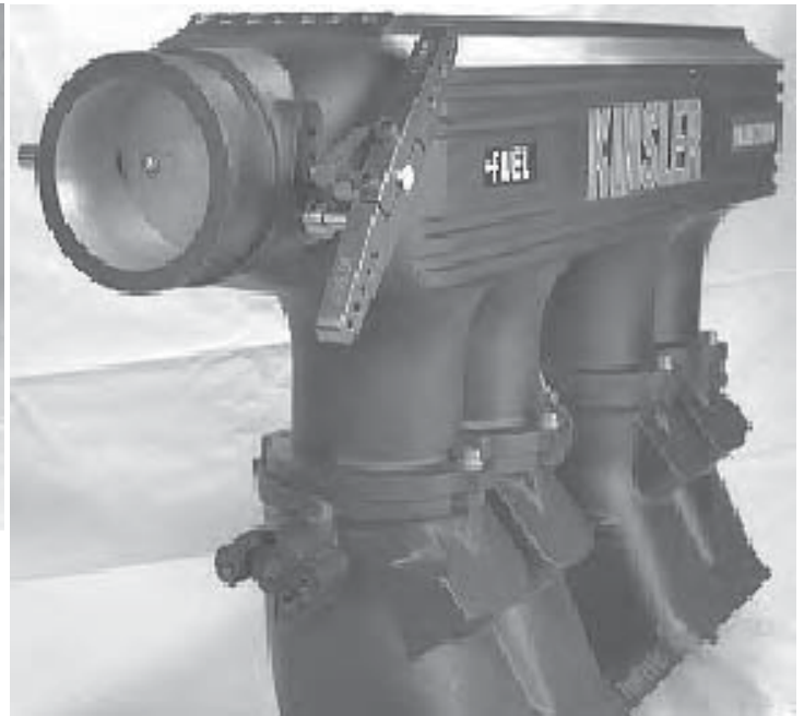
Log with 2.5" throttle plate and 2.5" runner outlets to manifold
