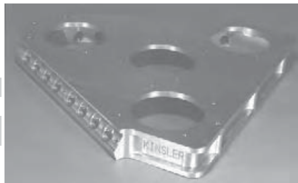
Throttle body adapter to go on top of PSI® supercharger
