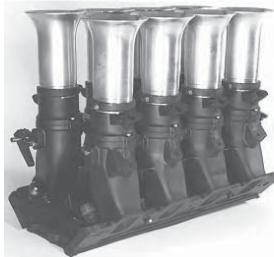
EFI injector bosses in the ramtube adapters
