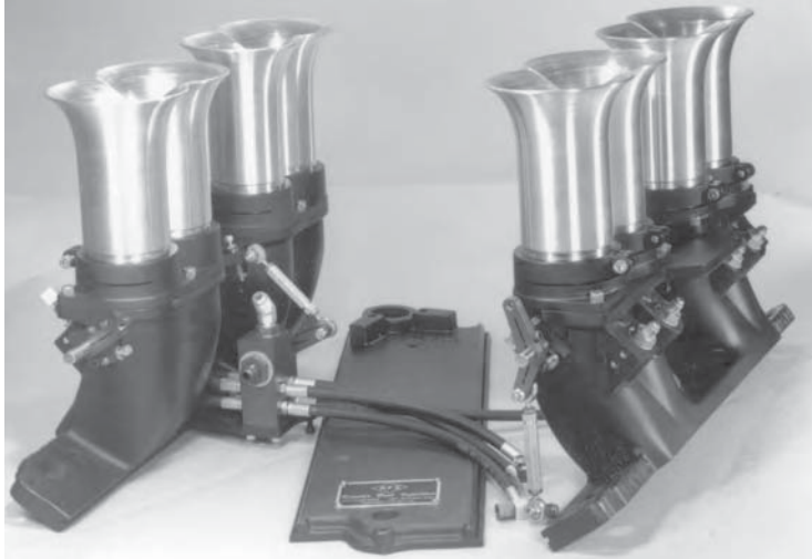
Constant flow fuel metering installed
