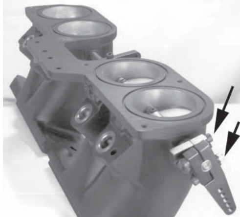
CORRECT Pulling arm installed next to throttle stop
